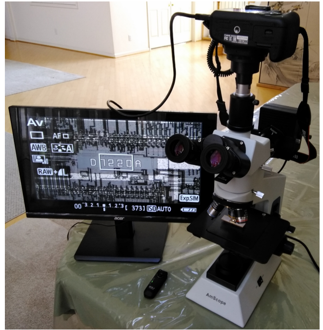
High Definition (1920 x 1080) Monitor and SLR Digital Camera Connected by HDMI Cable
