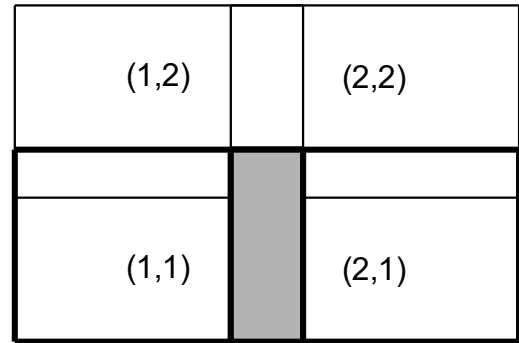
Four Adjacent Stacks ((1,1), (2,1), (1,2), & (2,2)) Overlapped 30% Horizontally & 35% Vertically
