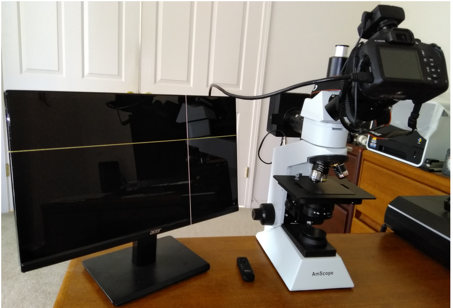
Screen Division Indices are Attached on Monitor TV to Clearly Define the Captured Area to be Overlapped
