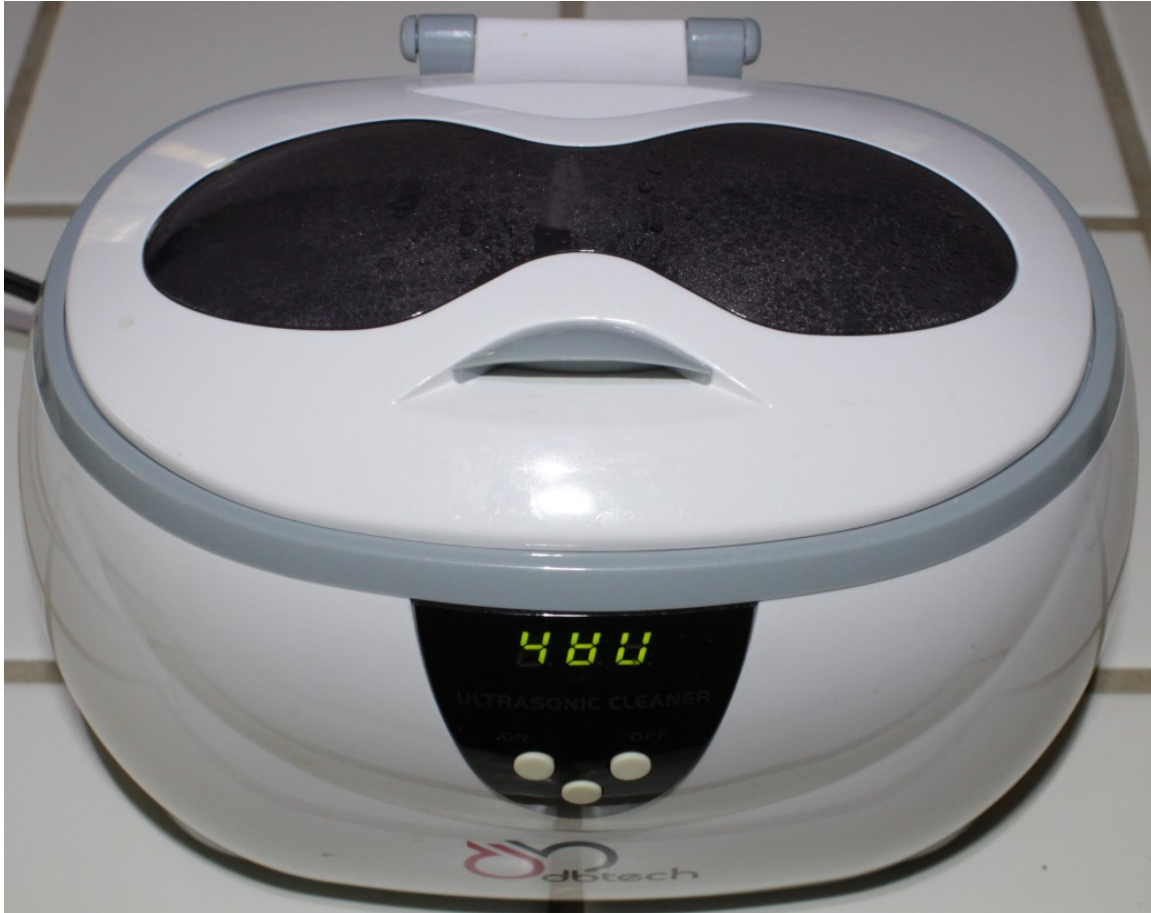
Ultrasound Cleaner (Cleaning Time of 480 Seconds Specified)
