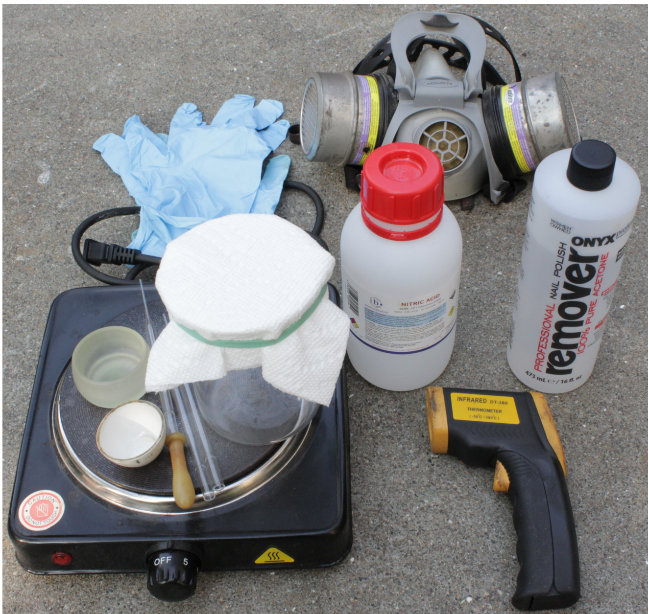
2.5 ml Pipettes, 400 ml Beaker, 15ml Crucible, 1 kW Hot Plate, Half-face Respirator, 70% Nitric Acid, 100% Acetone, Infrared Digital Thermometer, 5 mil Nitrile Gloves
