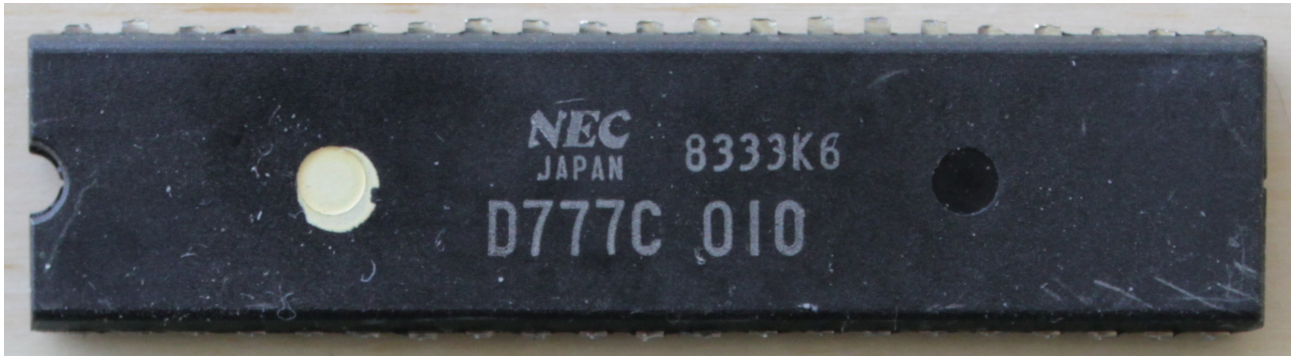
NEC \mu PD777C (Television Game LSI I Designed, 42 pins)
