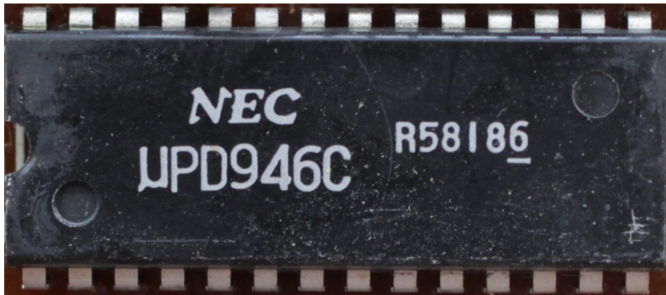
NEC \mu PD946C (8 Digits Desk-top Calculator LSI with One Memory, 28 pins)
