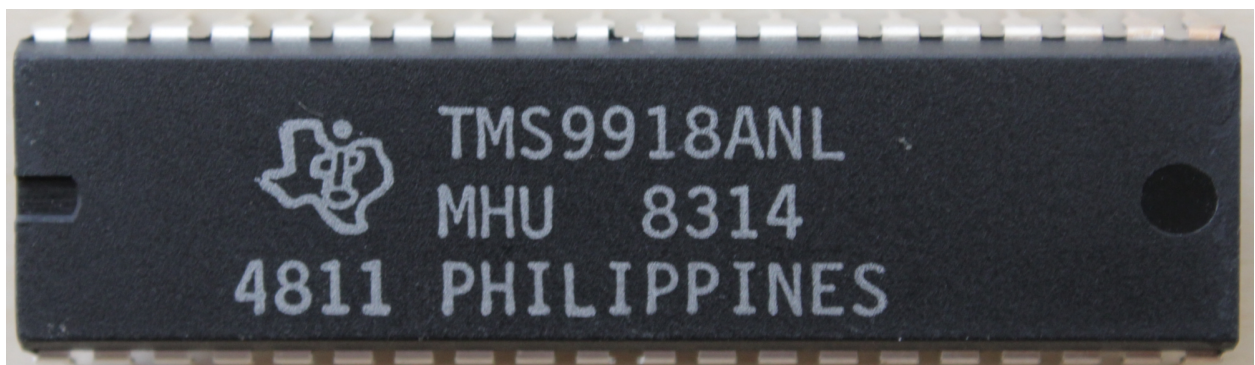
Texas Instrument TMS9918A (Video Display Processor for Sprite Control of Television Game, 40 pin)
