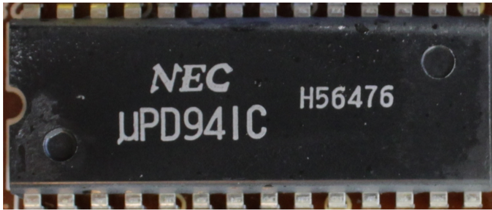
NEC \mu PD941C (8 Digits Desk-top Calculator LSI with No Memory I designed, 28 pins)
