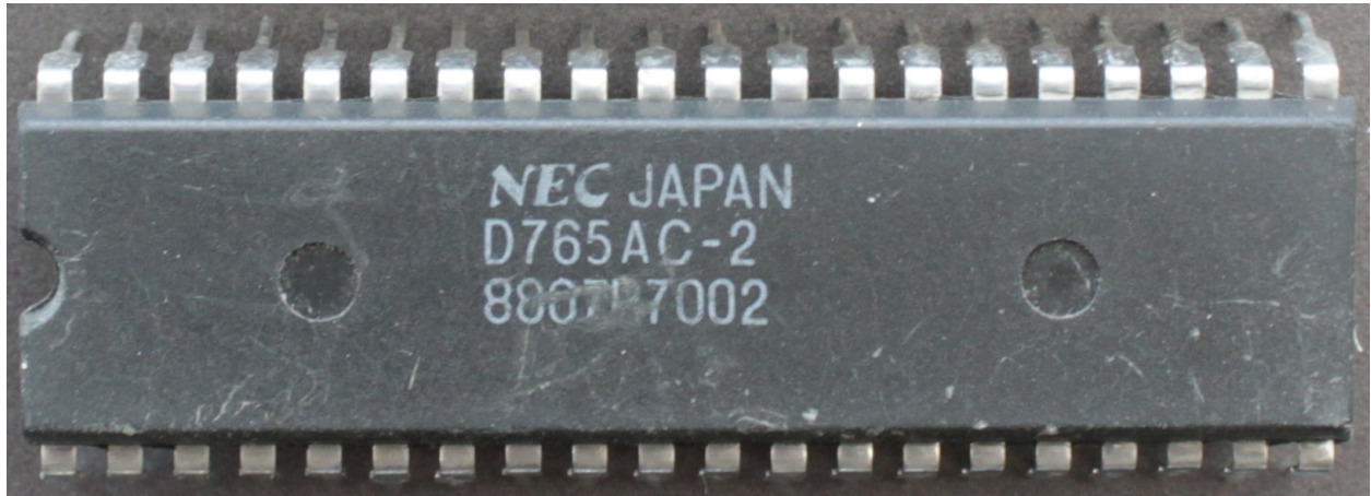
NEC \mu PD765AC (Floppy Disk Controller, 40 pins)
