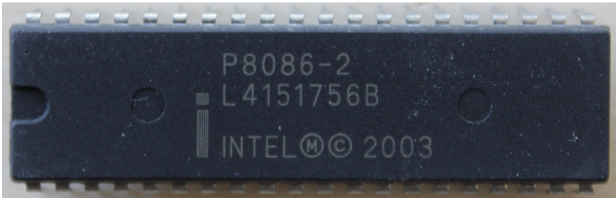
Intel 8086 (16 bit CPU, 40 pins)
