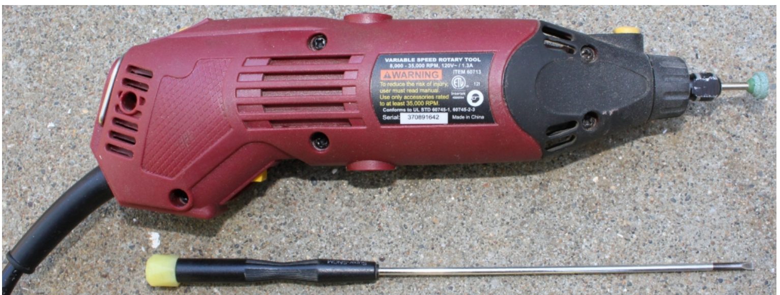
Decapsulation by Rotary Tool & Flat Head Precision Screw Driver Succeeded
