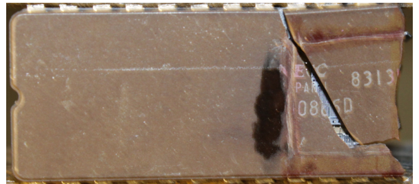
Made Scribe on Four Sides, then Hit Center Punch at Lower Right Corner (Was not exact corner..)
