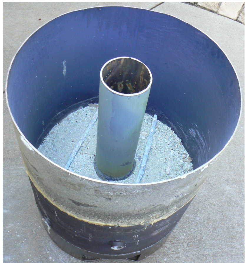
Sediments, Scales & Anode Rod Deposited in the Tank
