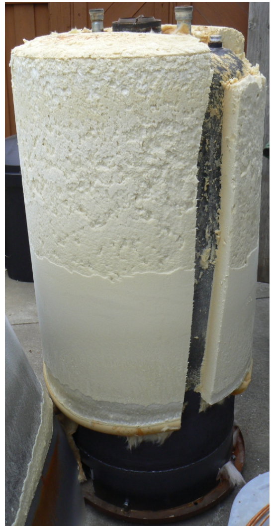
2" Thick Heating Insulator
