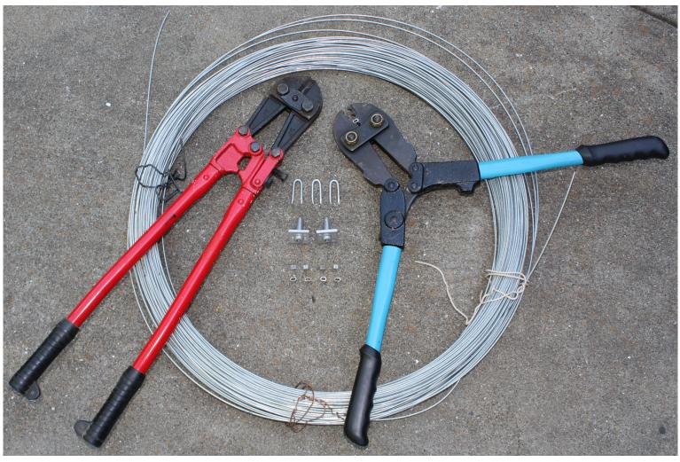
10 Gauge Galvanized High-tensile Wire, Wire Cutter, Single Barbed Staples, Internal Spring-loaded Wire Clamps, Wire Sleeves, & Crimp Tool
