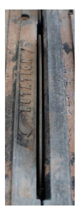
Saw Blade is Cooled by Water Rotating through Water Tank Stored under the Deck Plate
