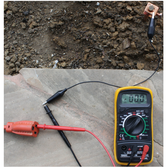
Neutral vs Earth (0V; equivalent voltage)
