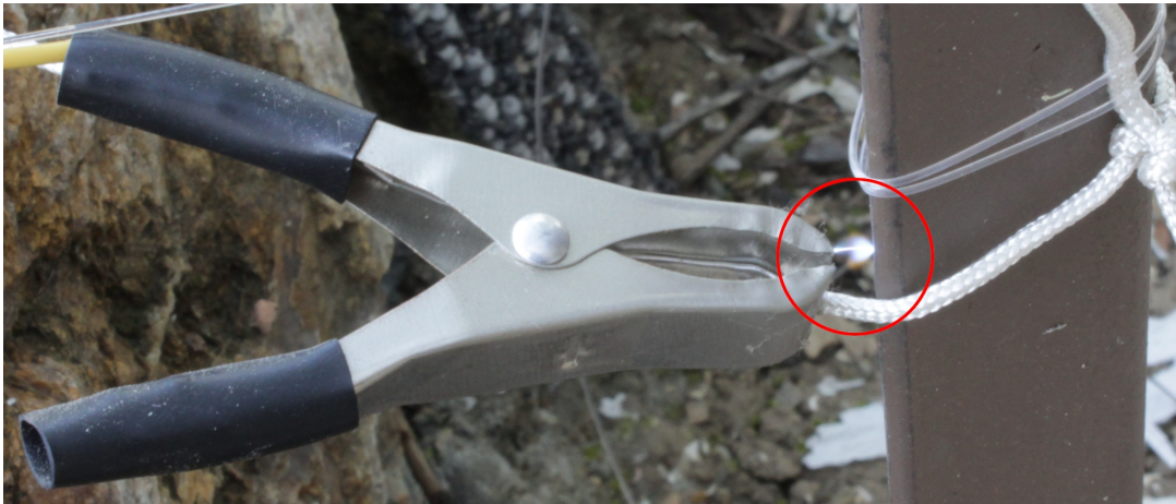
Spark test (Sparked successfully between high voltage pulse wire and iron stay bar hammered into ground)
