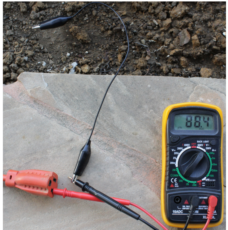
Hot vs Quasi Earth Rod (< 120V; higher resistance)
