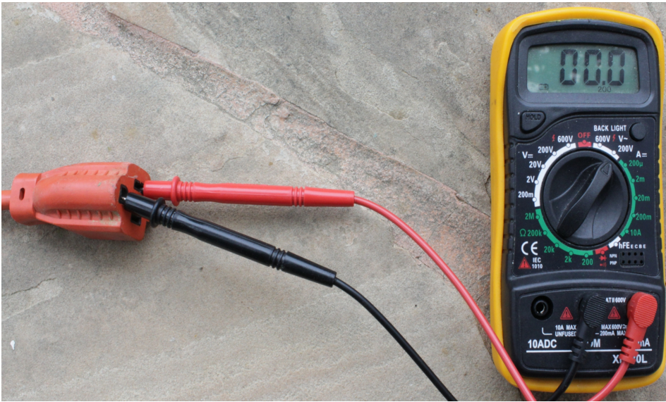
Neutral vs Ground (0V; equivalent potential voltage)
