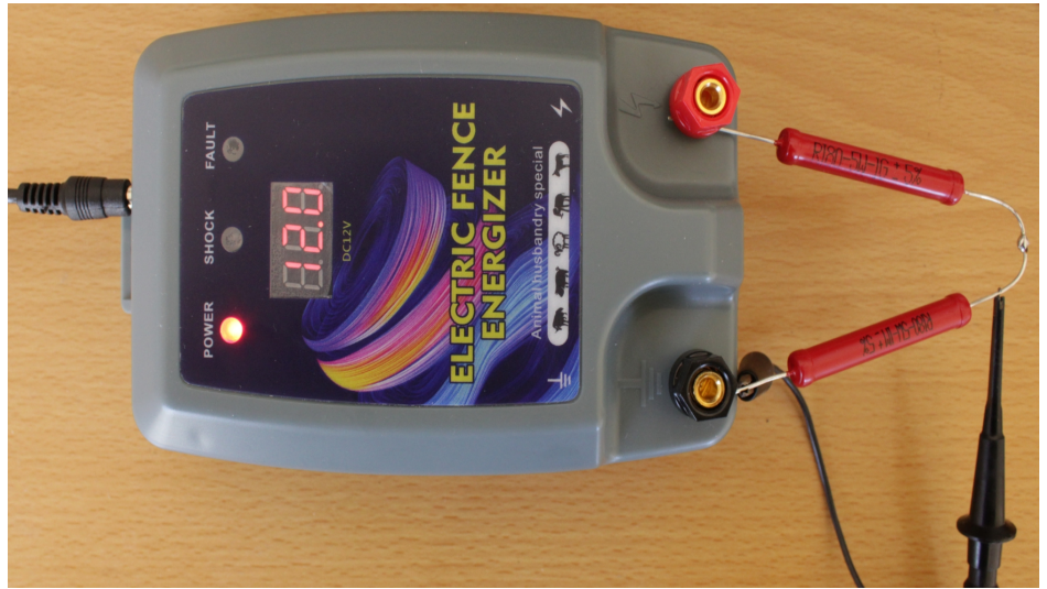
Working Electric Fence Energizer with external 1/1001 attenuator
