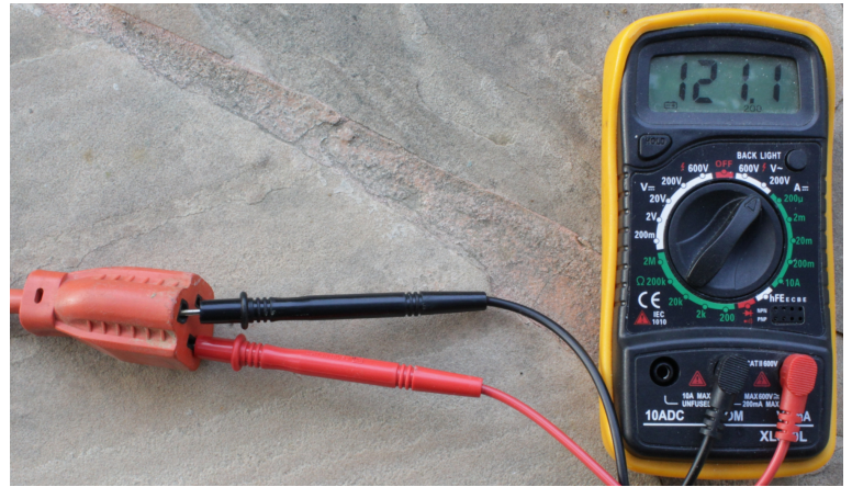
Hot vs Ground (AC 120V)
