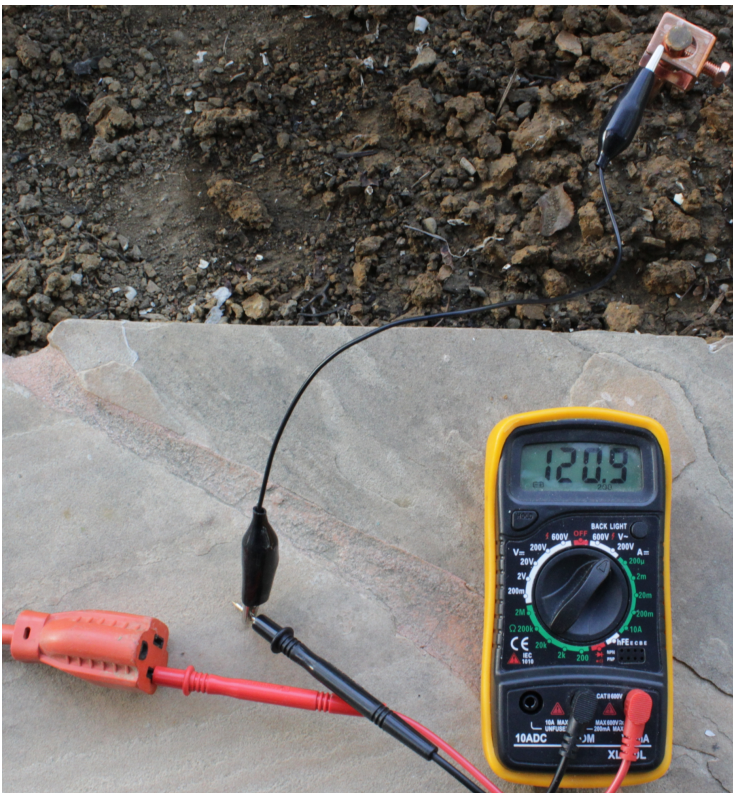
Hot vs Earth Rod (AC 120V; lower resistance)
