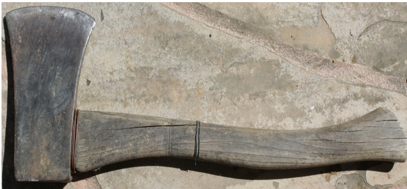
Hand axe used for hammering earth rod down to deep ground (around 4') efficiently
