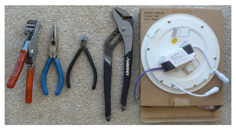
Wire Stripper, Long Nose Plier, Diagonal Cutter, Groove Joint Plier, 6" LED Light Module with Rectifier
