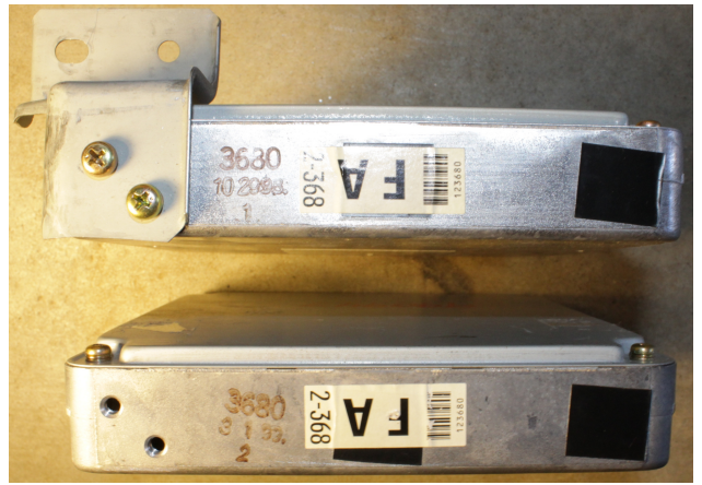
New ECM with bracket (Up) & Old ECM (Down)
