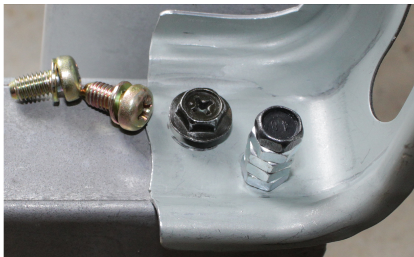
Hex bolts replaced Philips head bolts factory used to make it easy detaching/attaching ECM next time
