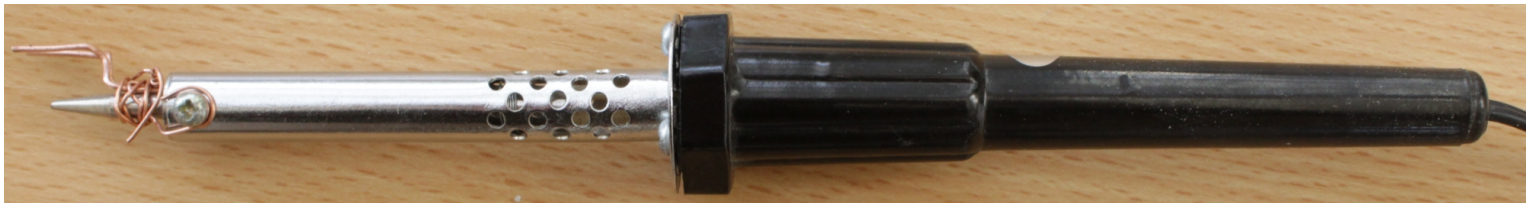
8 pin SOIC IC Remover I made
