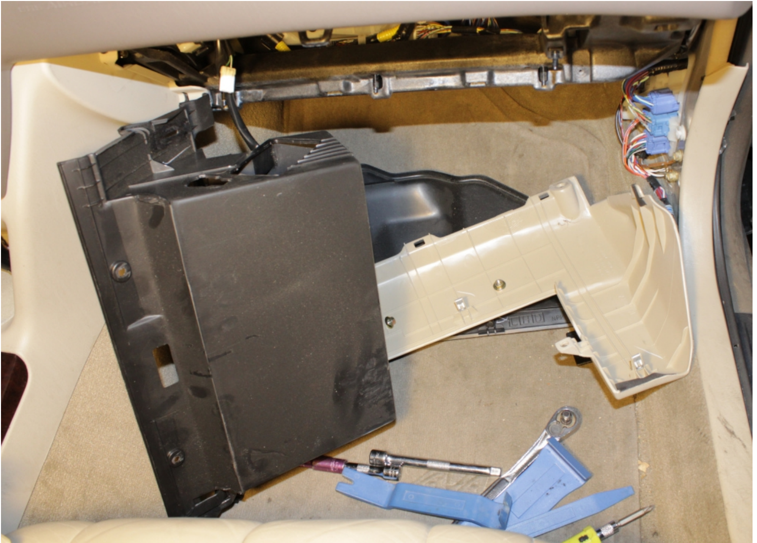
Removed glove box and etc.
