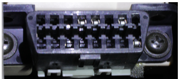
OBD2 Connector on Avalon (P13 has no female tab)
