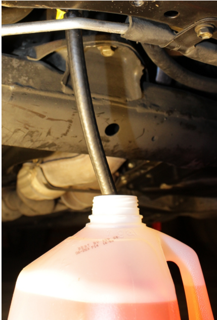
Draining coolant from radiator
