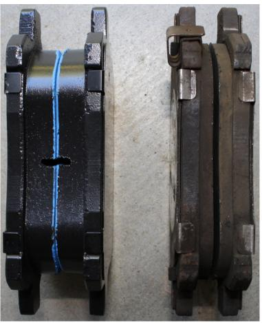
Thick New & Thin Old Brake Pads
