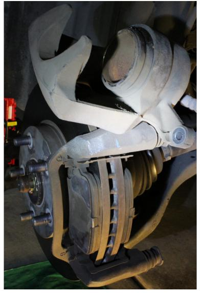
Brake Pads Exposed (Up; Brake Caliper Detached)
