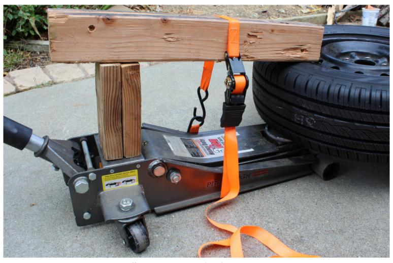
Efficient Low Cost Beads Release System
