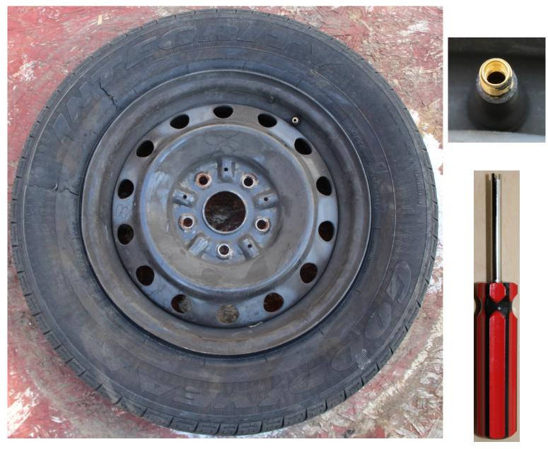
Old Tire with Cracks, Valve Core Driver
