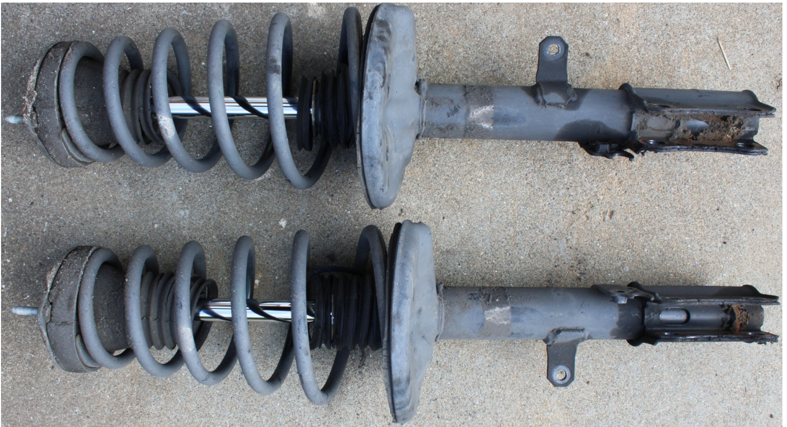
Old strut assemblies (rear right (upper) & rear left (lower); Tab position differs) removed
