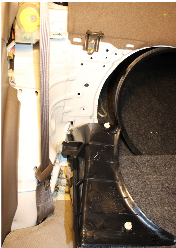
Plastic black trim behind the backrest removed
