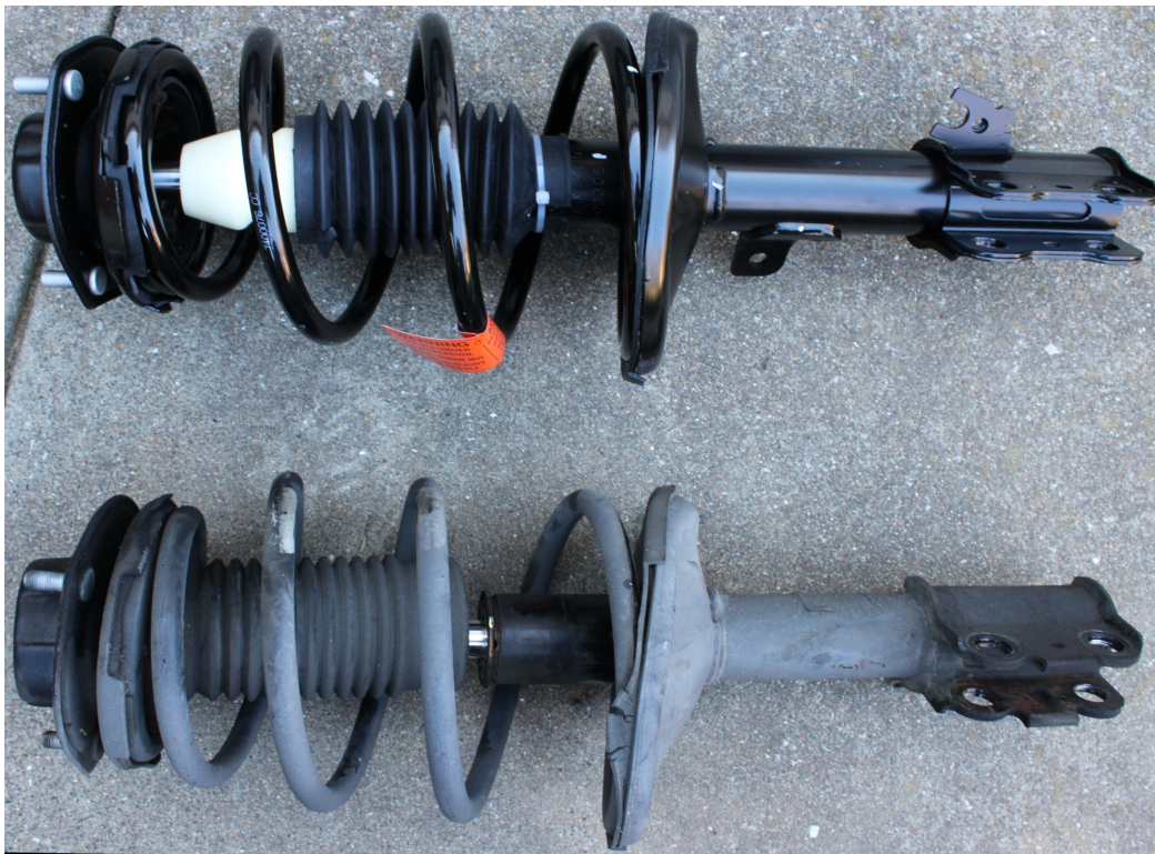
Front strut assembly New (upper) & Old (lower) Coil spring 3.5 turns (Front strut assembly) instead of 5.5 turns (Rear strut assembly)
