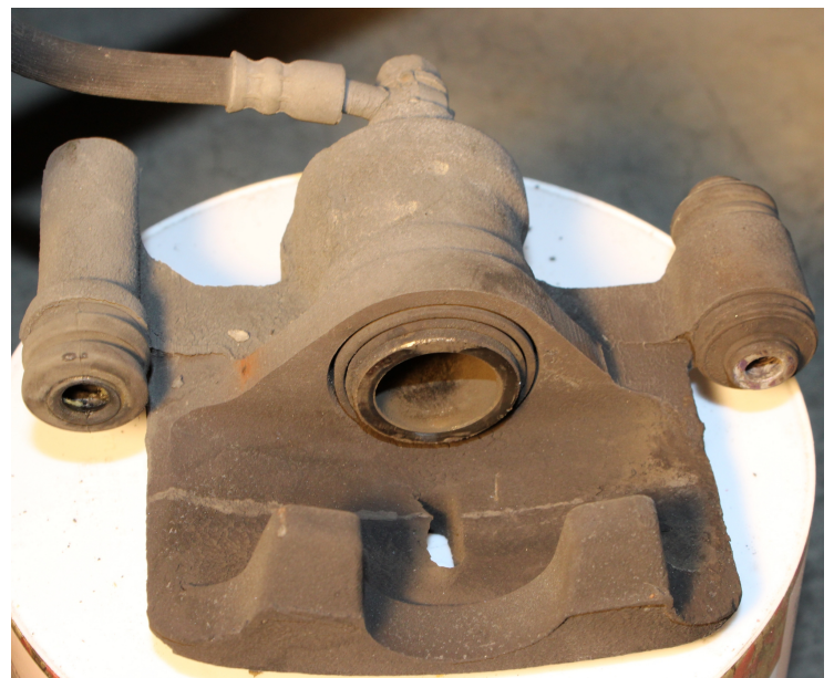
Brake caliper detached temporarily To re-install, piston must be pushed in by wrench.
