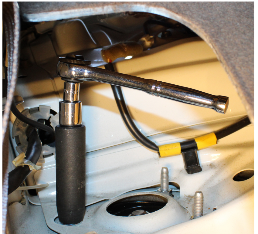
Using 1/4" small ratchet with 1/4" to 3/8" to 1/2" adapters
