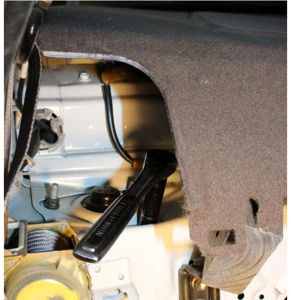
Brown plastic trim removed, top strut assembly nuts exposed supporting a board by a 2x4 lumber (lower right)
