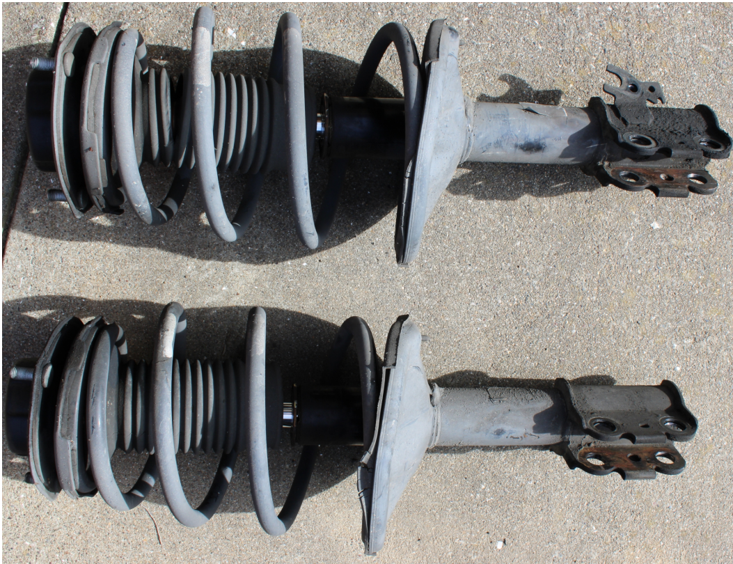
Old strut assemblies (front right (upper) & front left (lower); Tab position differs) removed
