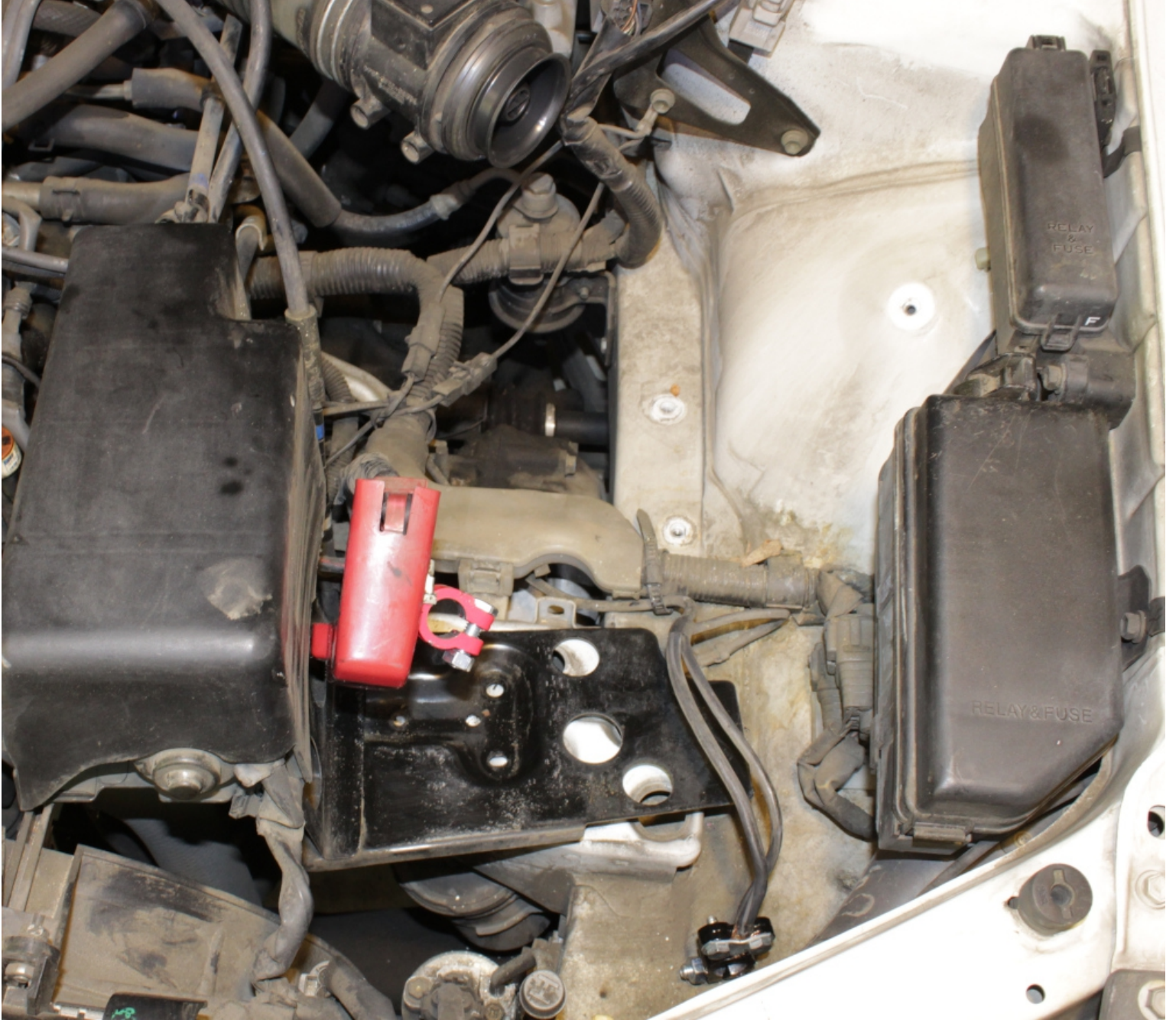
Preparation (Remove battery, Air filter housing,,,,)
