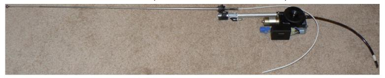
New Antenna with long antenna drive cable
