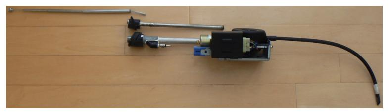
Broken Antenna (Antenna drive cable broke & shortened)
