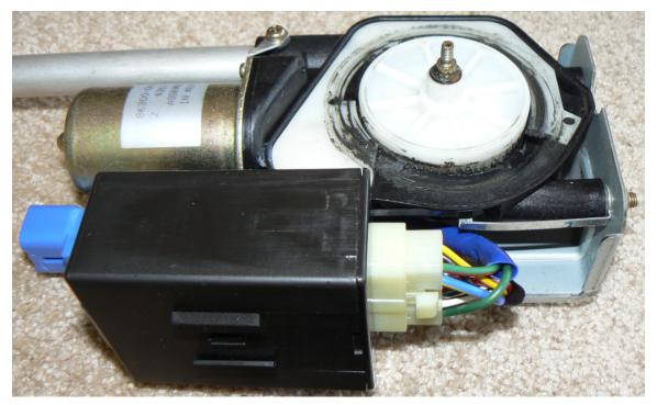
Powered Antenna Motor & Gear Unit
