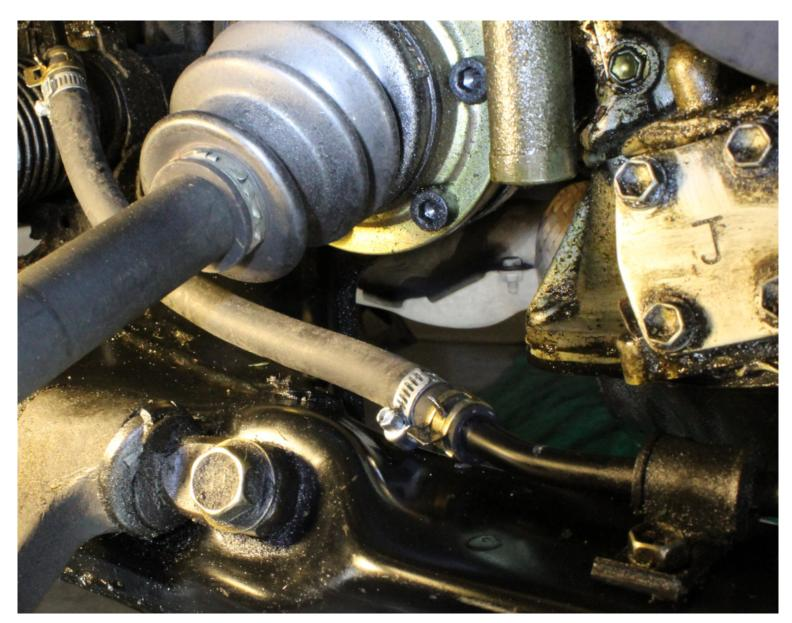
Power Steering Pump Pressure Feed Tube Replaced
