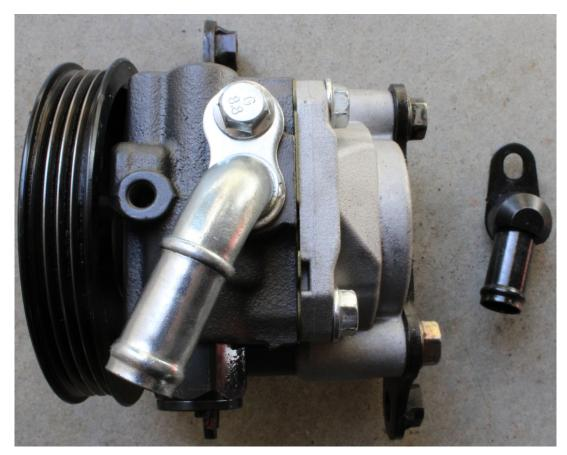
Return Hose, Bracket, New Power Steering Pump Assembled with Parts
