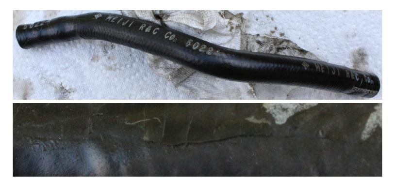
Old Power Steering Pump Pressure Feed Tube with Crack
