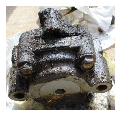
Old Power Steering Pump Fully Being Drenched by Power Steering Oil
