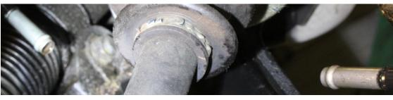
Old Power Steering Pump Pressure Feed Tube Removed
