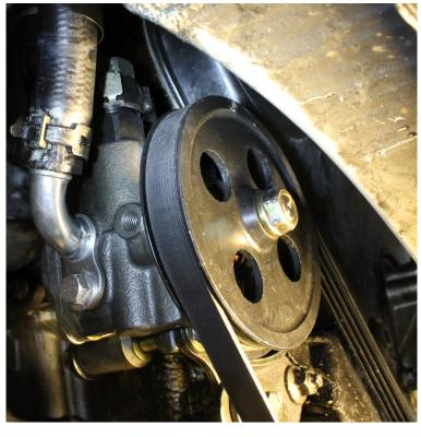
Replaced (Clean; No Oil Leak)
