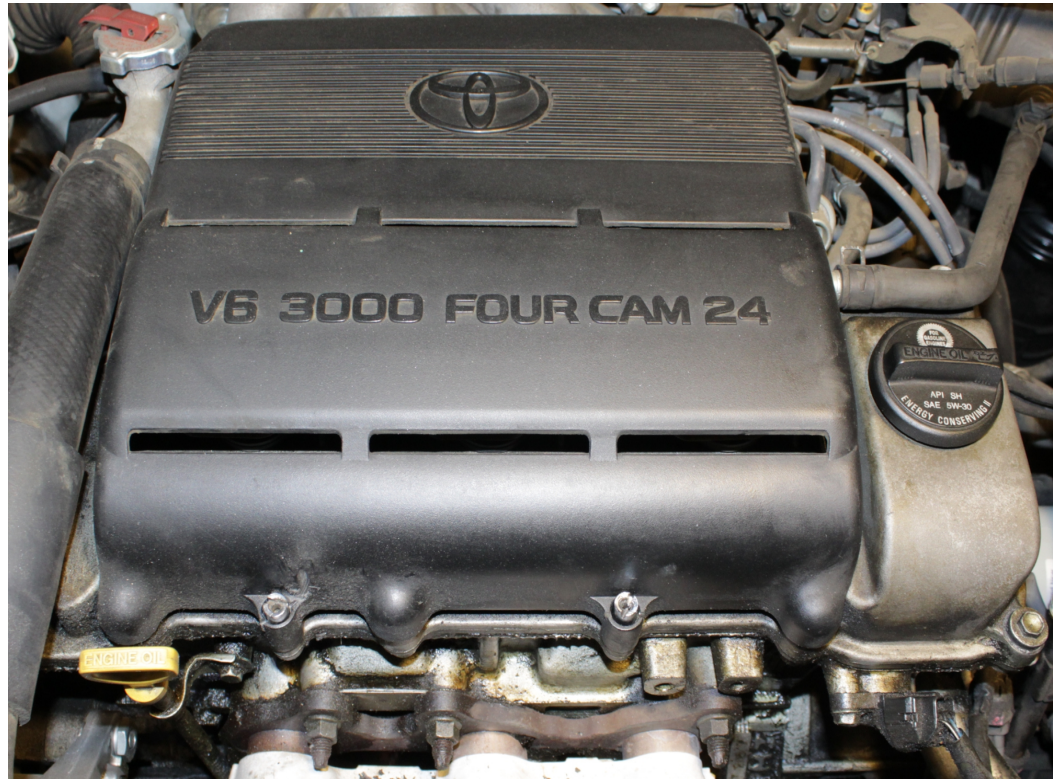
Plastic Engine Cover fastened by two stud nuts
