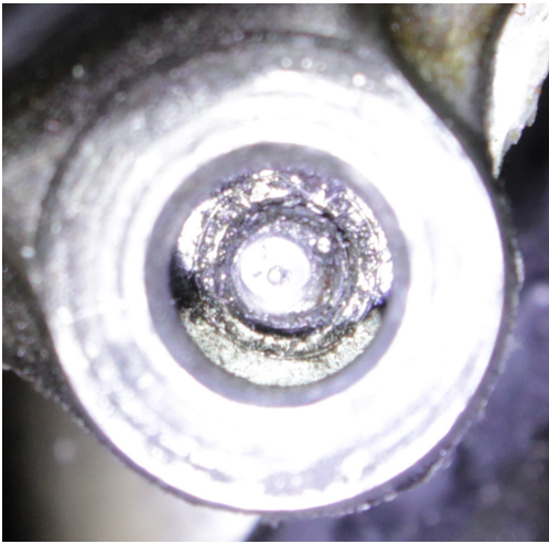
Center punch to get precise center
