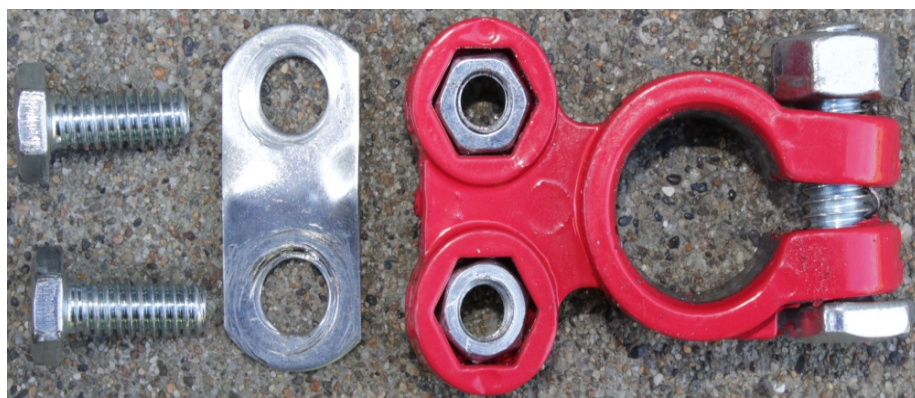
Good looking problematic battery terminal sold in market (Before filing off red paint on surface)
