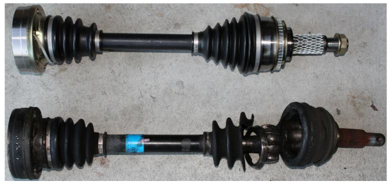
New Drive Axle with CV Joint (Top) & Old Drive Axle with Broken CV Joint (Bottom)
