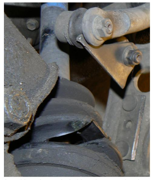
Broken Stabilizer Link Set Bracket (Right) & Broken CV Joint Sleeve (Bottom)
