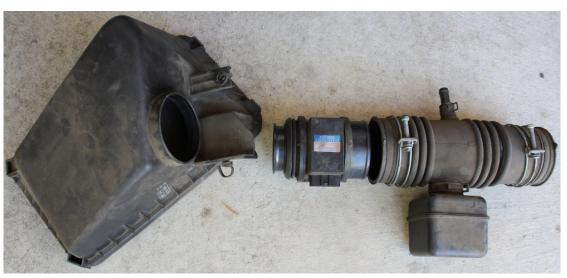
Mass air flow sensor itself is working well (No need to replace).
