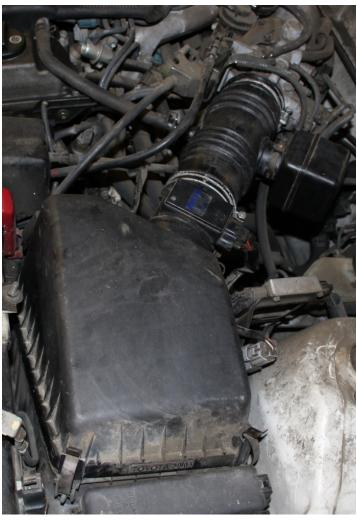
Replaced Air Filter (Bottom) & Tube (Center Right)
