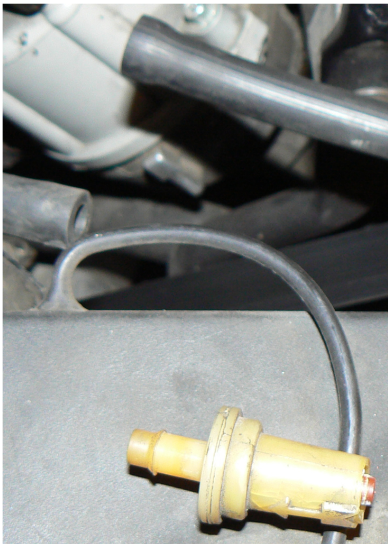
Broken Plastic Coupling
