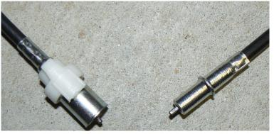
New Cable (Left to speedometer, Right to cable linkup)
