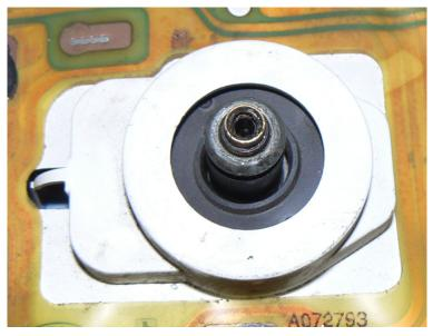
Cable Receptacle on New Instrument Cluster
