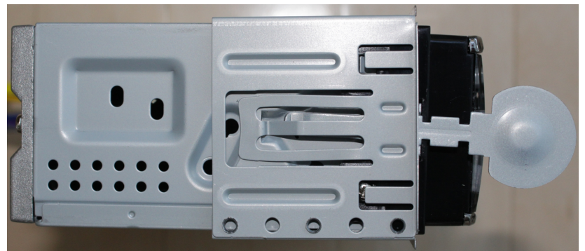
Radio must be able to be detached from Mounting collar by handling two Bracket keys
