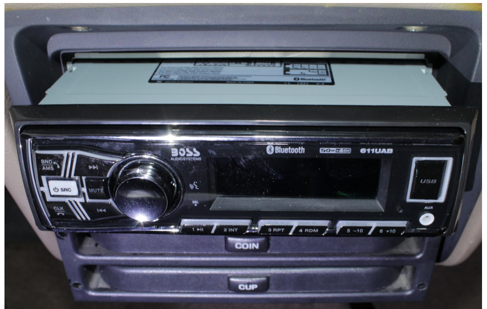
Wire connection completed by soldering Restoring radio & accessory into DIN (Deutsches Institut für Normung)
