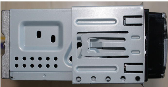
Radio must be able to be detached from Mounting collar by handling two Bracket keys
