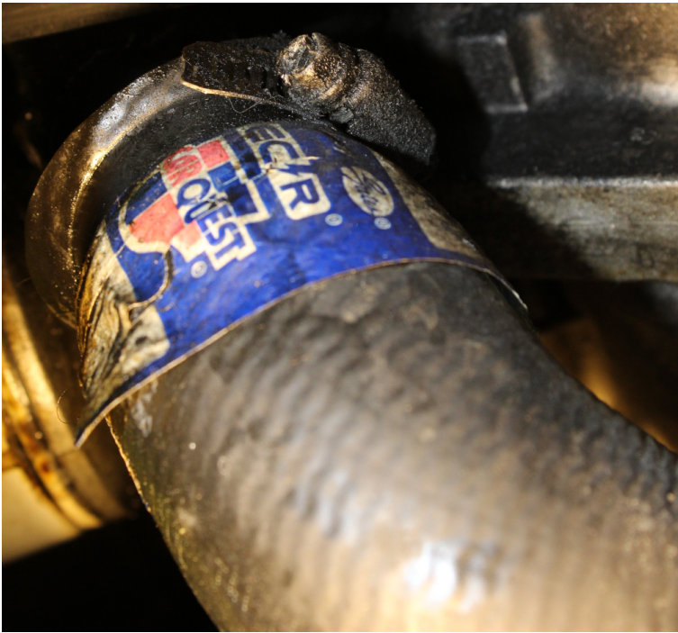
Old Radiator Hose Installed
