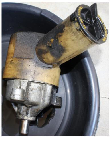
Power Steering Pump Removed (No Bracket)
