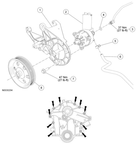
Power Steering Pump & Pulley
