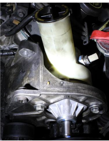
New Power Steering Pump Installed (No Pulley)
