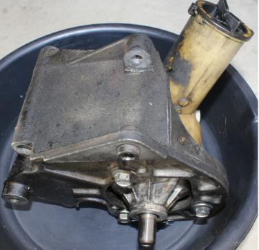
Power Steering Pump Removed (with Bracket)
