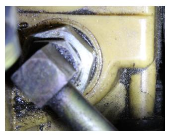
Crack on Plastic Return Hose Inlet (Design Flaw)
