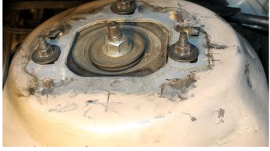
Top mounting nuts fastened tightly
