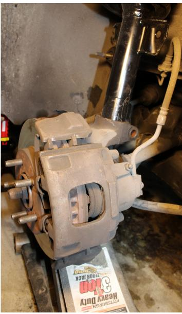
Strut assembly & steering knuckle engazed
