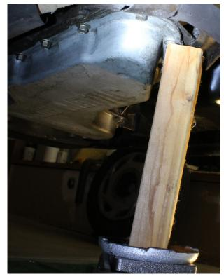
Pushing up the Engine through Oil Pan
