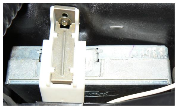
Engine Control Module Support
