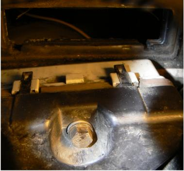
Rear (Left) & Front (Right; with Connector) Engine Control Module Bay
