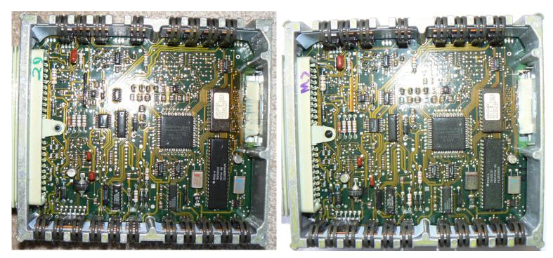
Old (Left) & New (Right) Engine Control Module (Parts Side)
