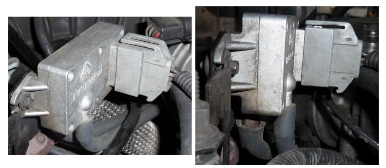
EGR (Exhaust Gas Recirculation) Pressure Sensor Hose Deteriorated (Left side hose)
