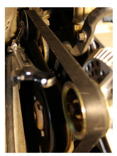
Combined Wrench Technique Applied for Drive Belt Tension Release
