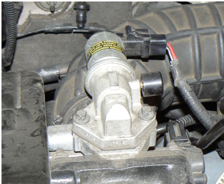
Old Air Flow Control Module Installed
