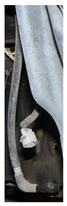
Fluid Outlet Connection & Pump Connector Removed
