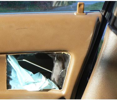
Making Window to Access Door Open/Close Mechanism
