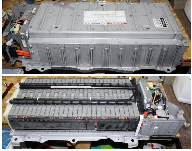
Main HV Battery Casing Removed (Battery modules are placed next to controller block, #1, to the far end, #28)
