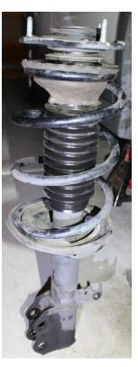
Assembled with New Boot, Dump Stop & Spring
