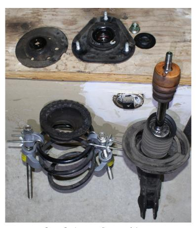
Strut Spring etc. Removed Apart
