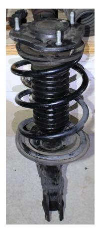
Assembled with New Boot, Dump Stop & Spring
