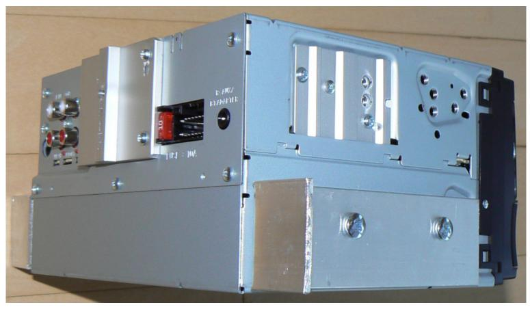
Mounting Tabs Newly Made (before making two holes at each back)
