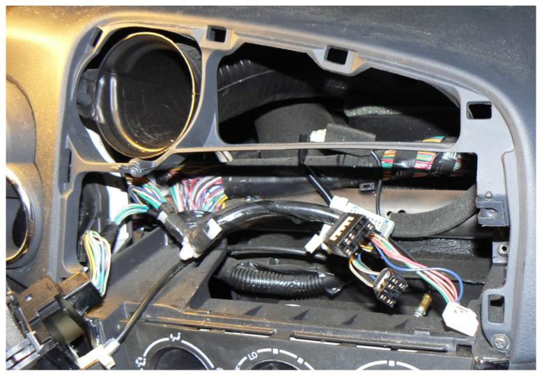
Old Car Stereo Removing from Console
