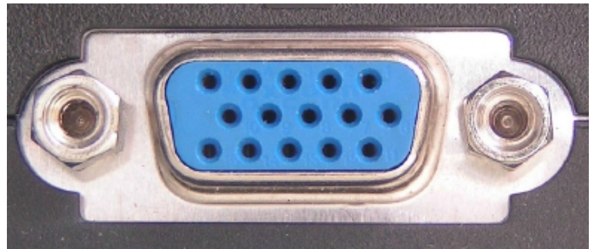
Female connector HD15S D-Sub (Both PC and monitor device implement)
