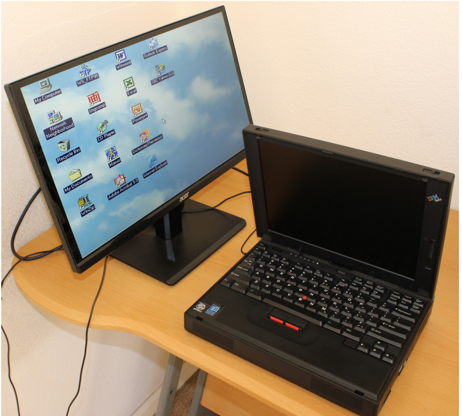
IBM ThinkPad 380XD VGA connector > "VGA to HDMI adapter" > LCD monitor TV (Resolution: 800 x 600 SVGA)
