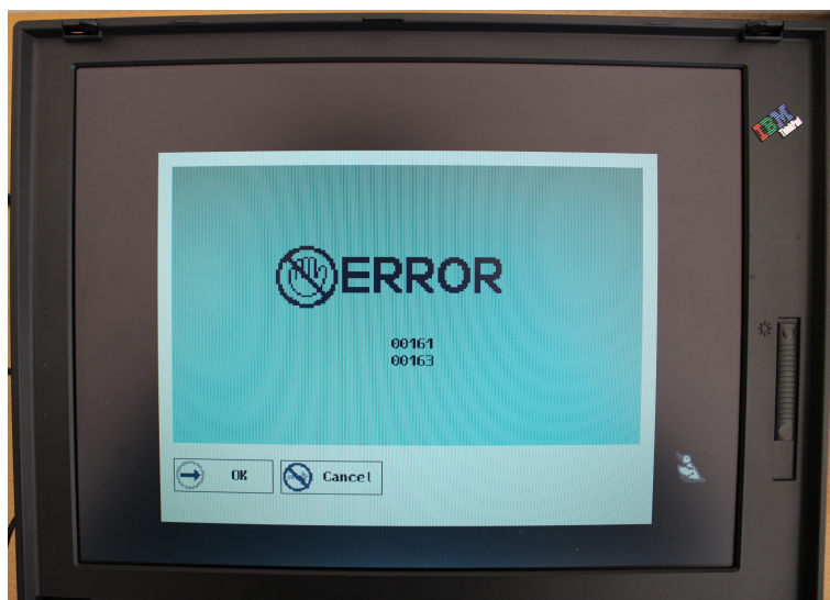
If CMOS battery discharges, error message appears
